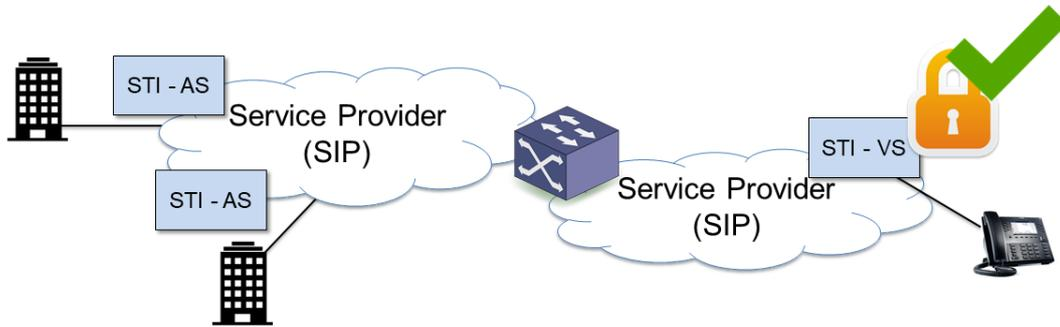
**Figure 1: Mechanism for calls between users on SIP-based networks (Source: ATIS)**
