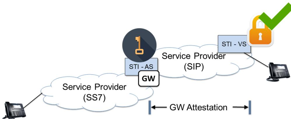
**Figure 2: Calls originating from SS7 networks and terminating on SIP-based networks (Source: ATIS)**
