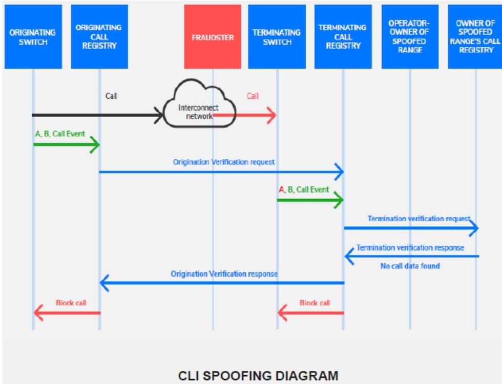
**Figure 9: CLI validation for CLI spoofing detection (Source: AB Handshake)**
