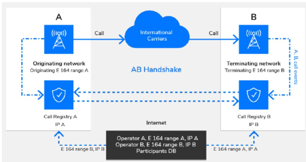
**Figure 10: AB Handshake Out-of-Band System Architecture (Source: AB Handshake)**
