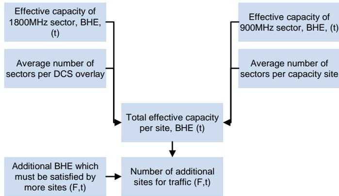
Figure A.5: Calculation of the number of additional sites required to satisfy BHE traffic requirements [Source: Analysys Mason]
