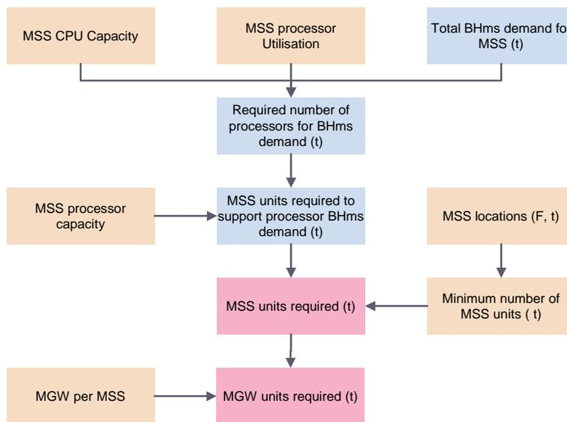
Figure A.31: Calculation of MSS units to support processing demand and MGW [Source: Analysys Mason]
