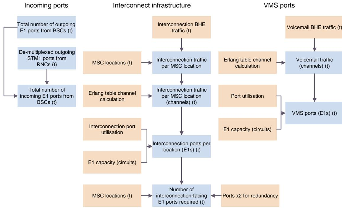
Figure A.12: Without a transit layer – calculation of MSC ports: BSC-facing ports, interconnect-facing ports, VMS-facing ports [Source: Analysys Mason]
