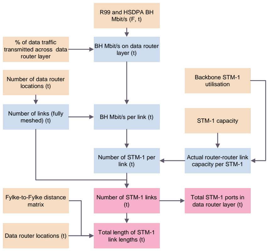
Figure A.35: Calculation of links between data routers in the packet-switch layer [Source: Analysys Mason]
