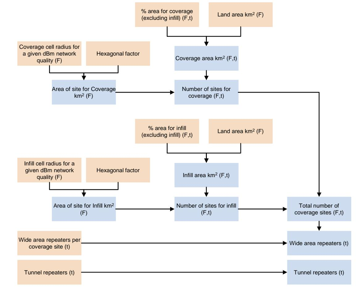
Figure A.1: 900MHz coverage network design [Source: Analysys Mason]
