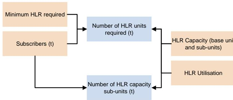
Figure A.18: HLR units calculation [Source: Analysys Mason]
