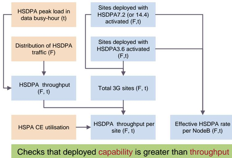
Figure A.26: Verification of sufficient HSPA deployment [Source: Analysys Mason]
