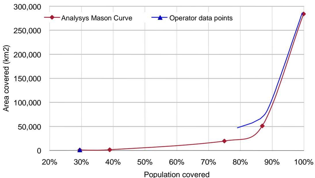
Figure G.1: Population and area coverage [Source: Analysys Mason, operator data]
