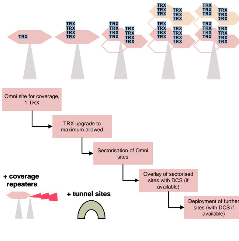
Figure 4.4: GSM radio network deployment
