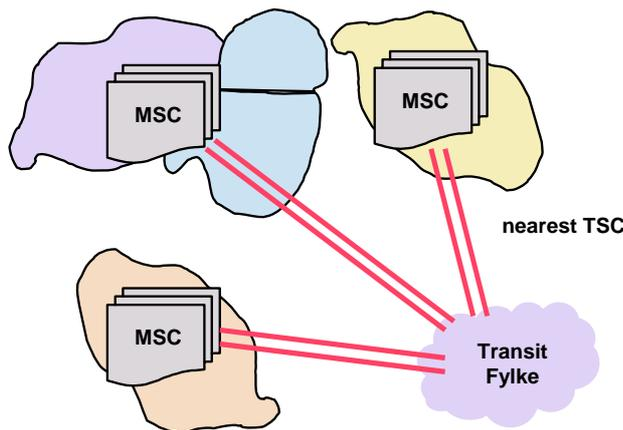
Figure 4.12: MSC–TSC transmission with the deployment of a transit layer [Source: Analysys Mason]
