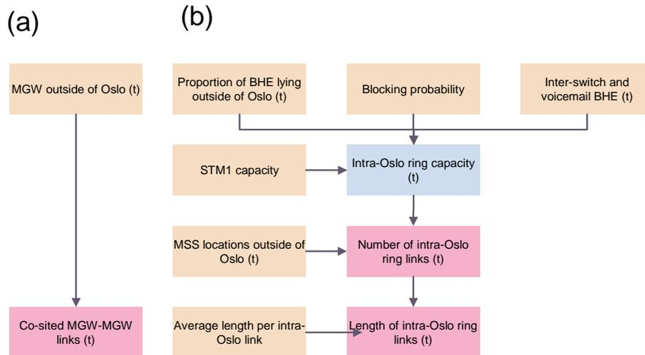
Figure A.33: Calculation of MGW–MGW links between (a) co-sited MGWs outside of Oslo and (b) MGWs outside of Oslo [Source: Analysys Mason]
