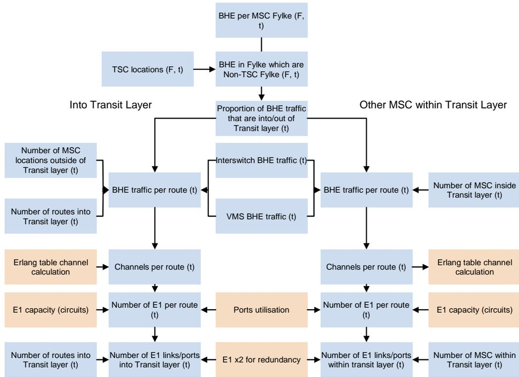
Figure A.14: With a transit layer – calculation of the number of inter-switch ports to the transit layer [Source: Analysys Mason]
