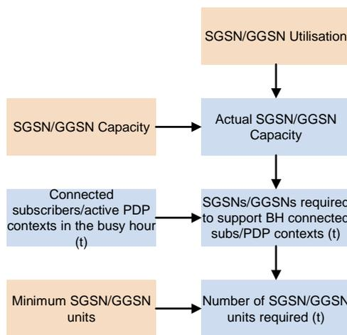
Figure A.20: SGSN and GGSN units calculation
