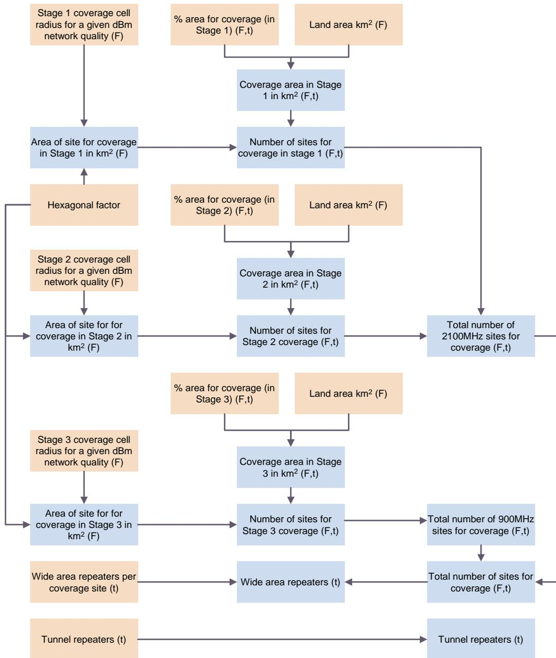
Figure A.21: UMTS coverage network design [Source: Analysys Mason]
