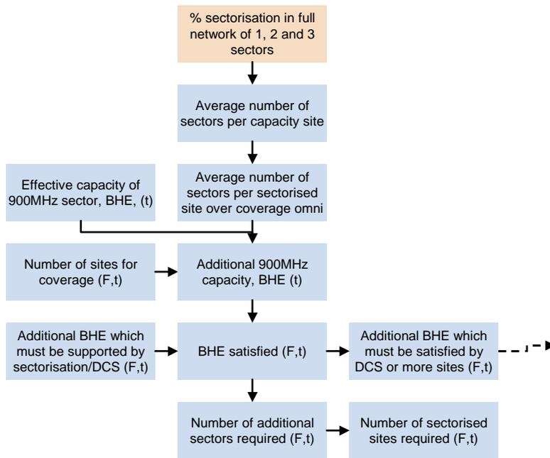
Figure A.3: Calculation of the capacity provided by sectorising coverage site [Source: Analysys Mason]
