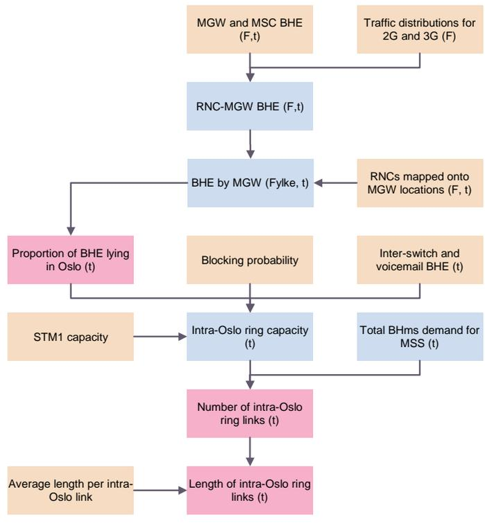
Figure A.32: Calculation of MGW-MGW links between Oslo sites [Source: Analysys Mason]
