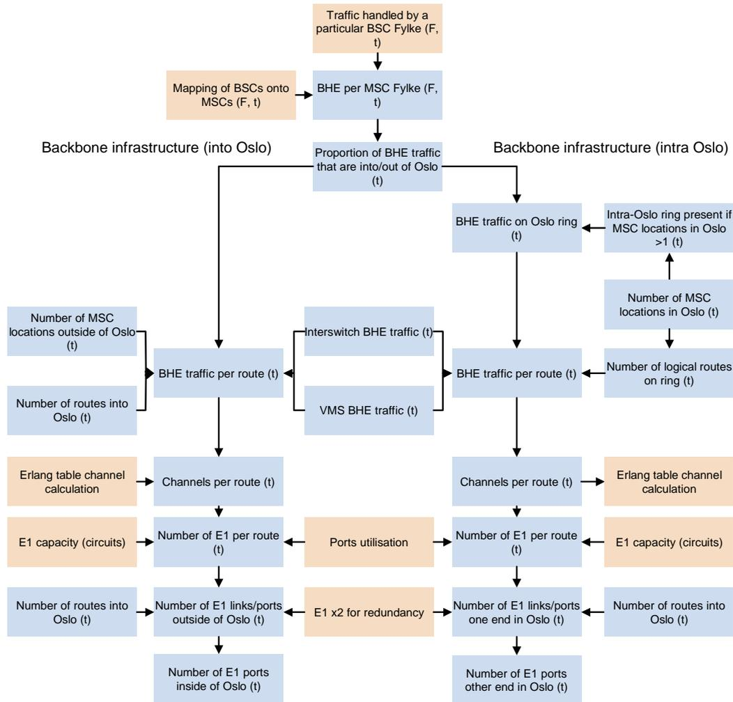
Figure A.13: Without a transit layer – calculation of the number of inter-switch ports [Source: Analysys Mason]
