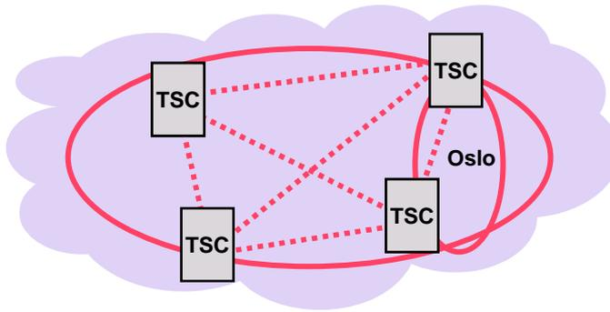
Figure 4.13: Fully meshed transit layer
