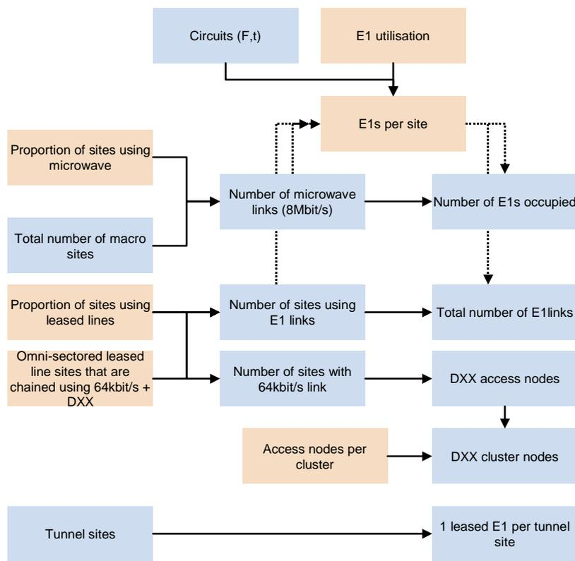
Figure A.7: Backhaul calculation [Source: Analysys Mason]
