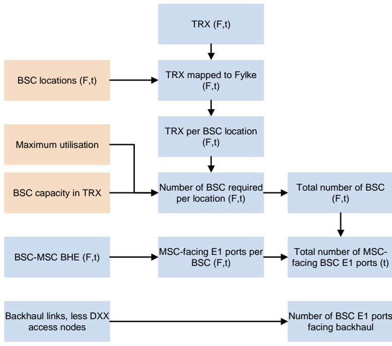
Figure A.8: BSC deployment [Source: Analysys Mason]
