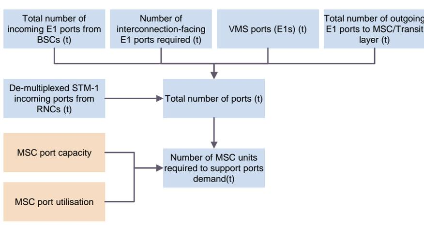
Figure A.15: Calculation of MSC units to support port demand [Source: Analysys Mason]
