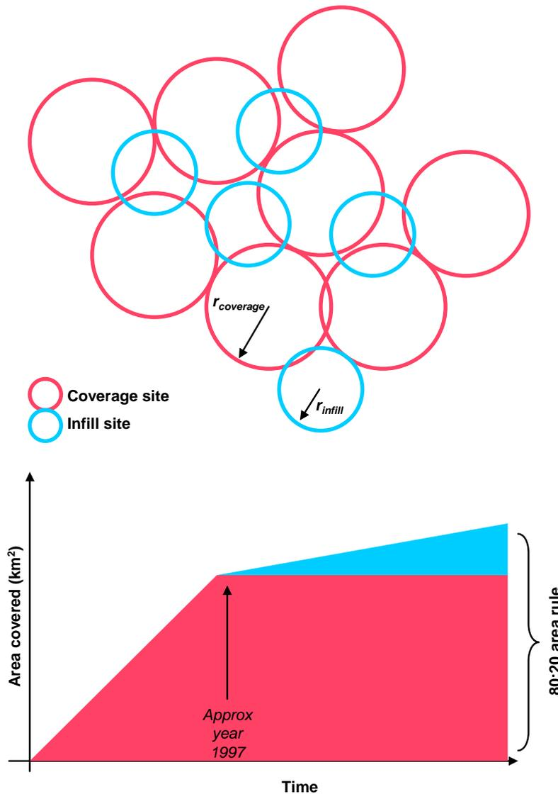
Figure 4.2: Wide-area GSM coverage and infill
