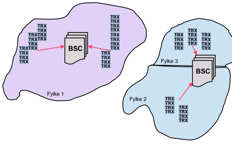
Figure 4.8: BSC deployment [Source: Analysys Mason]
