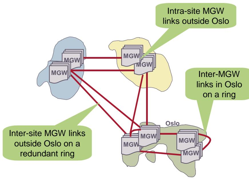
Figure 4.14: Modelled MGW-MGW links and ports [Source: Analysys Mason]
