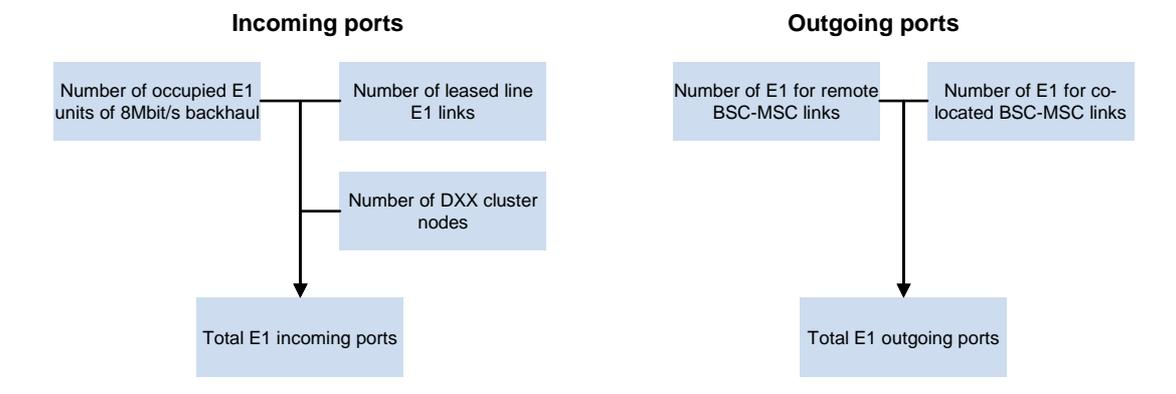
Figure A.10: Total incoming and outgoing ports for BSC [Source: Analysys Mason]
