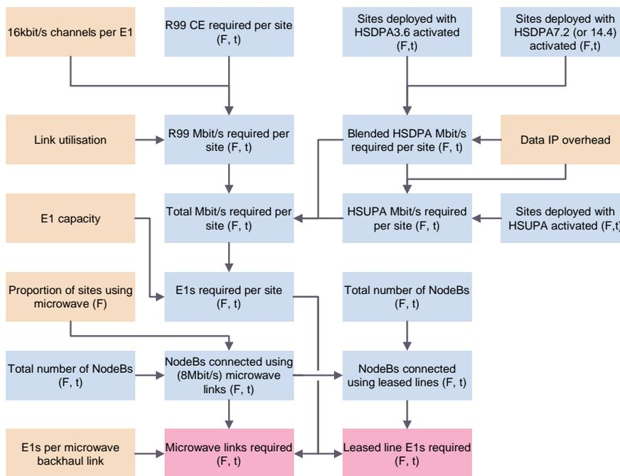
Figure A.27: UMTS backhaul calculation [Source: Analysys Mason]
