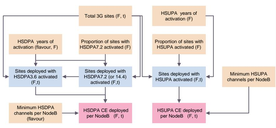
Figure A.25: HSPA channel element deployment [Source: Analysys Mason]
