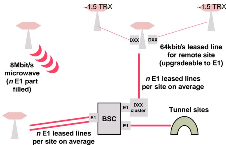
Figure 4.6: GSM backhaul configuration
