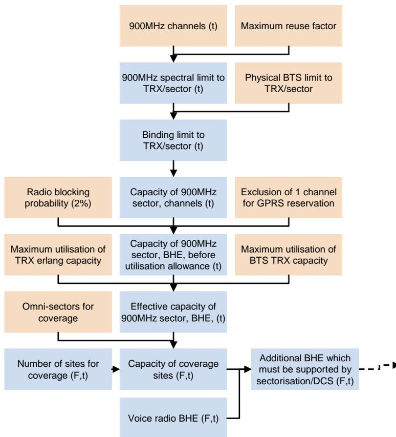
Figure A.2: Calculation of the BHE capacity provided by the coverage network [Source: Analysys Mason]
