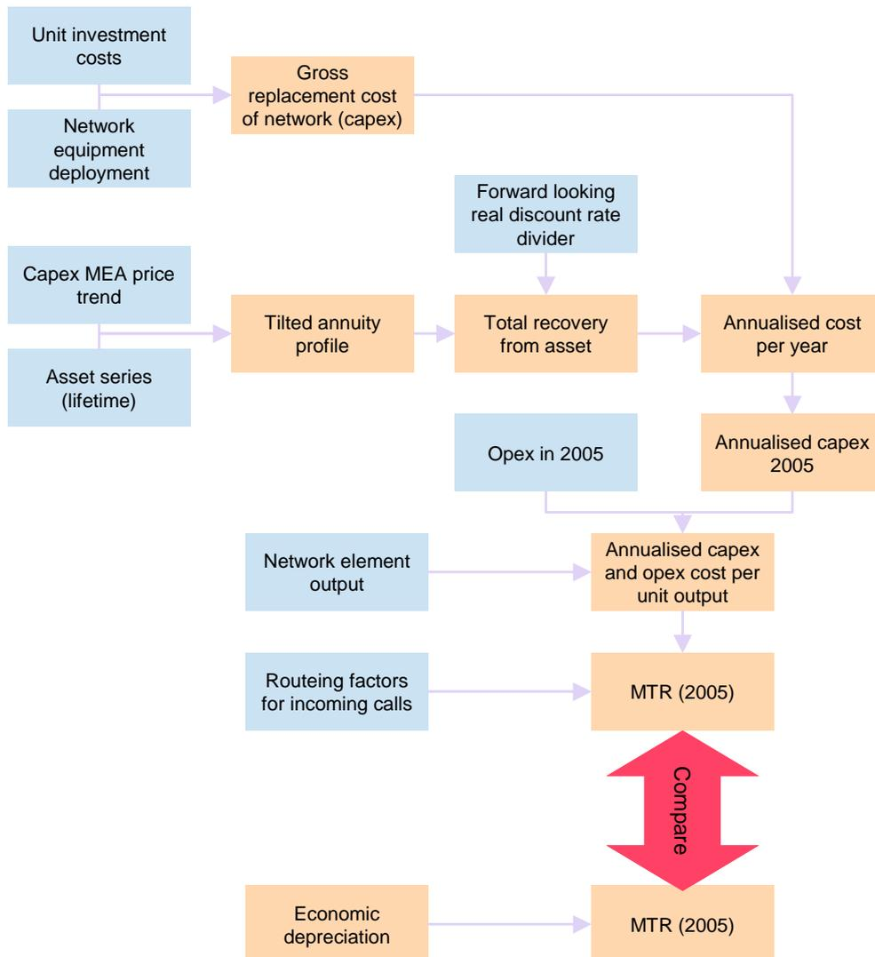
Figure 6.4: Tilted annuity calculation [Source: Analysys Mason]
