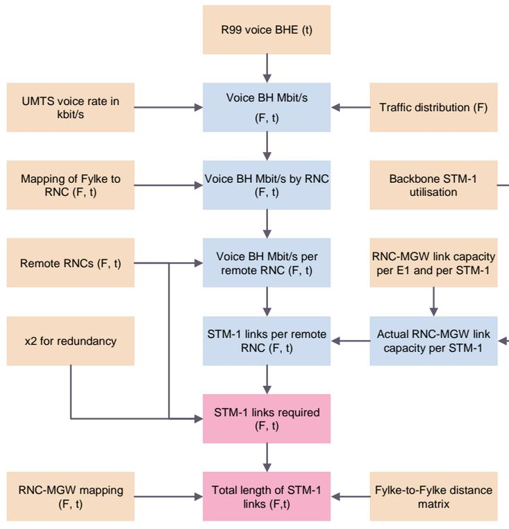
Figure A.34: Calculation of RNC-MGW links [Source: Analysys Mason]
