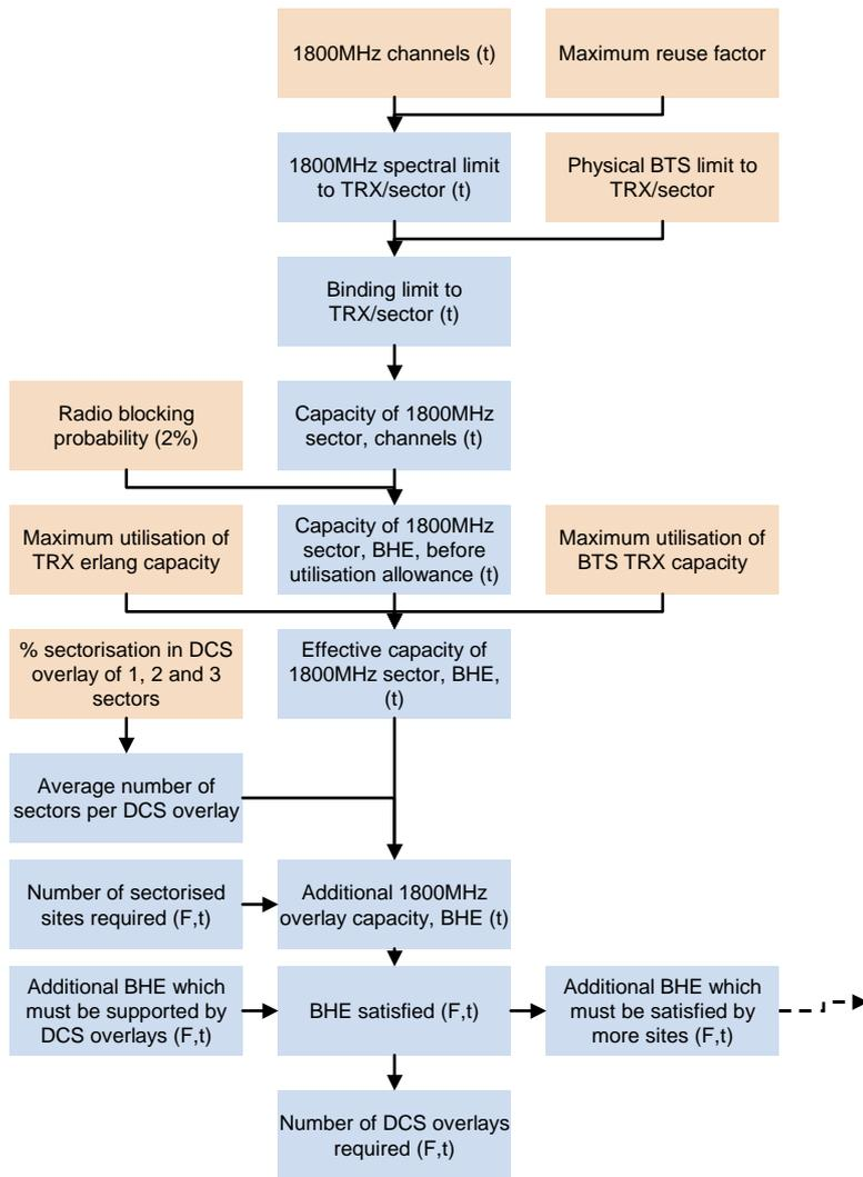
Figure A.4: Calculation of the capacity provided by overlaying coverage sites with DCS1800MHz spectrum [Source: Analysys Mason]
