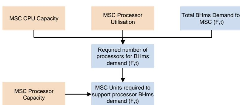
Figure A.11: Calculation of MSC units to support processing demand
