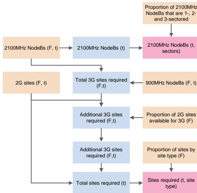
Figure A.23: Total site requirements [Source: Analysys Mason]
