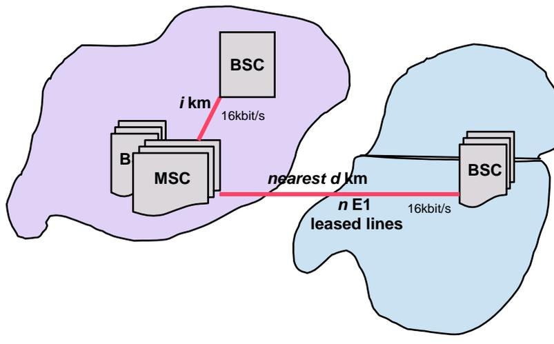
Figure 4.9: BSC–MSC transmission for remote BSCs [Source: Analysys Mason]
