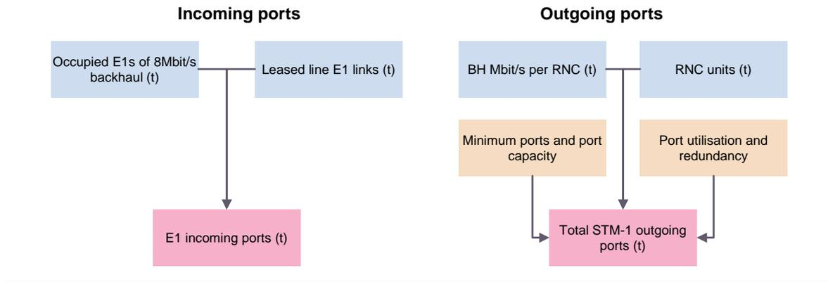
Figure A.30: Total incoming and outgoing ports for RNC [Source: Analysys Mason]
