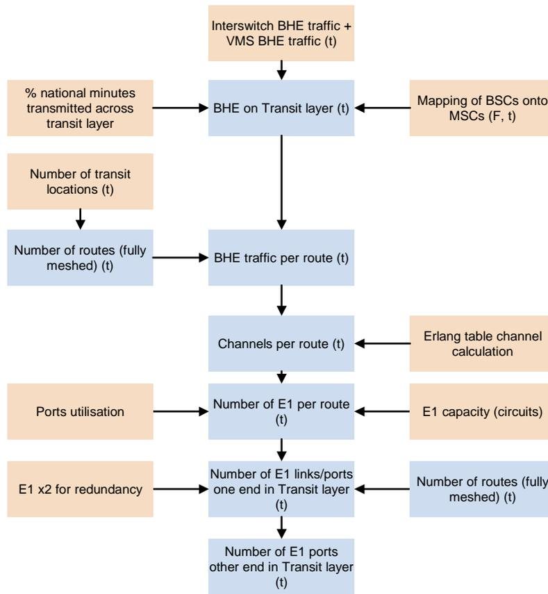
Figure A.17: Total TSC–TSC links for a network with transit layers
