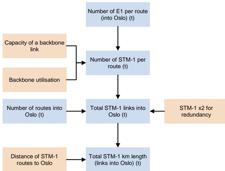
Figure A.16: MSC–MSC links for a network without transit layer [Source: Analysys Mason]
