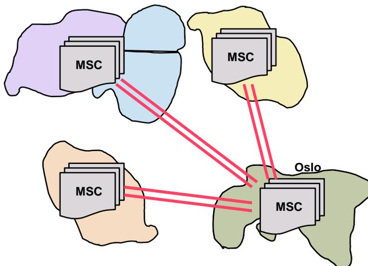
Figure 4.10: MSC–MSC transmission (no transit layer) [Source: Analysys Mason]
