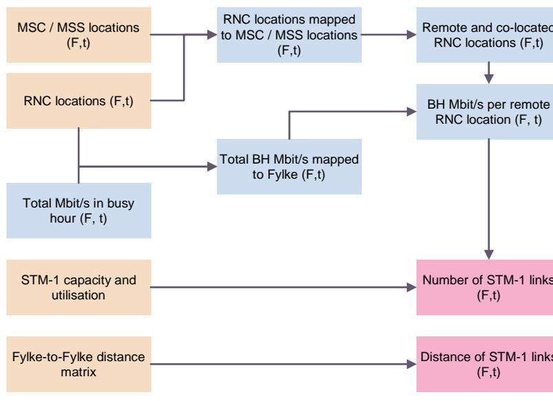
Figure A.29: RNC–MSC remote transmission in the legacy core network
