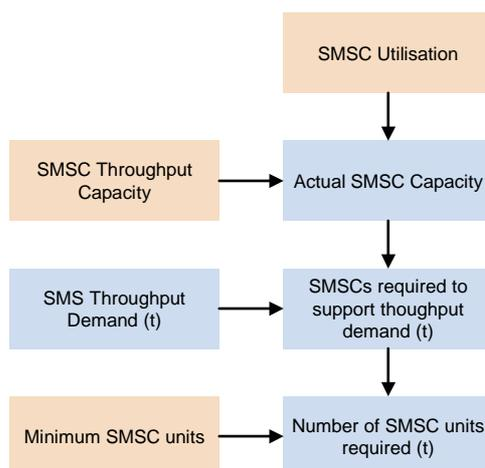
Figure A.19: SMSC units calculation [Source: Analysys Mason]
