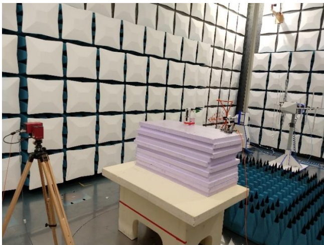
HF59D with Attenuator DG20_G10 under test
