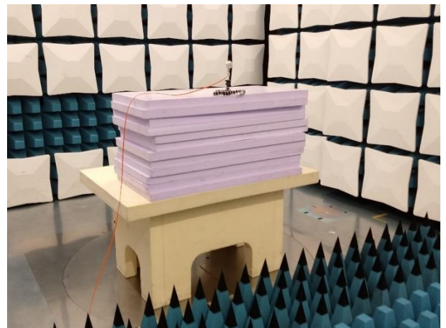
Field probe LSProbe 1.2 for calibration of electromagnetic field
