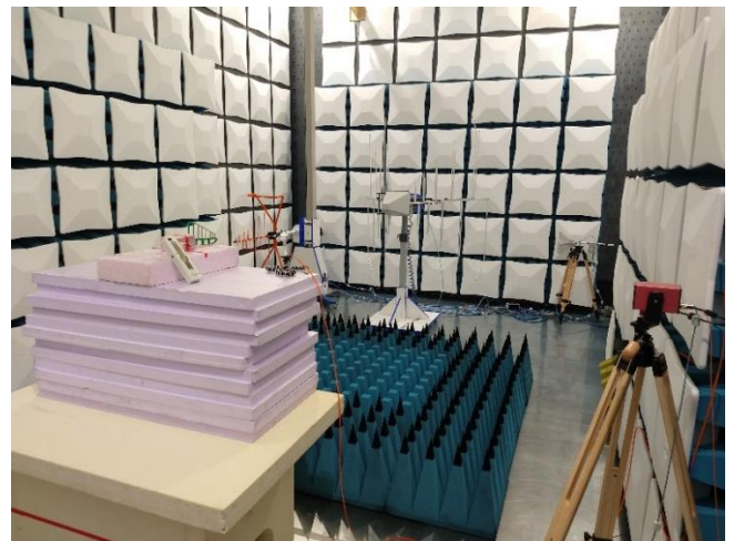
HF35C with Attenuator DG20_G10 under test
